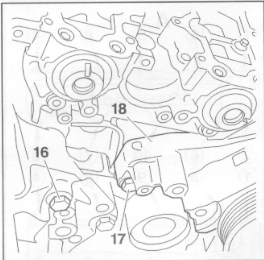
Fig : B1DP132C Remove the screws (16) and (17). Move the bracket (18) clear of the cylinder head.
